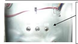
Your machine also has three circuit breakers inside the locked control panel door (which is also the cash box for 4202 and 4203 models). These breakers protect the computer board from an electrical short circuit by the ozone generator, fans or heating element during operation.
