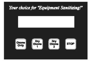
The 4201A model has four (4) buttons for its operation. The ozone only button will start the ozone "only" cycle. Ozone will be introduced into the cabinet for 12 minutes (16 minutes for DeconZone) and then an ozone reduction cycle will run from 1 to 8 minutes (1 to 12 minutes for DeconZone) depending on the ozone level within the machine. At the end of reduction, if the cabinet's ozone level is at the safe limit, the ozone sensor inside the cabinet will allow the magnetic lock to release.
